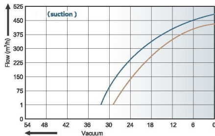
Performance Curve of GB Series Vortex Air pump (for reference only and not for testing basis)
